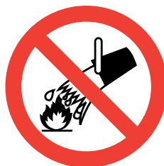
Do not extinguish with water
